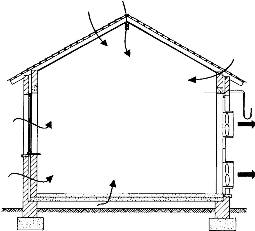
Figure 1 - Pressurisation measurement.
