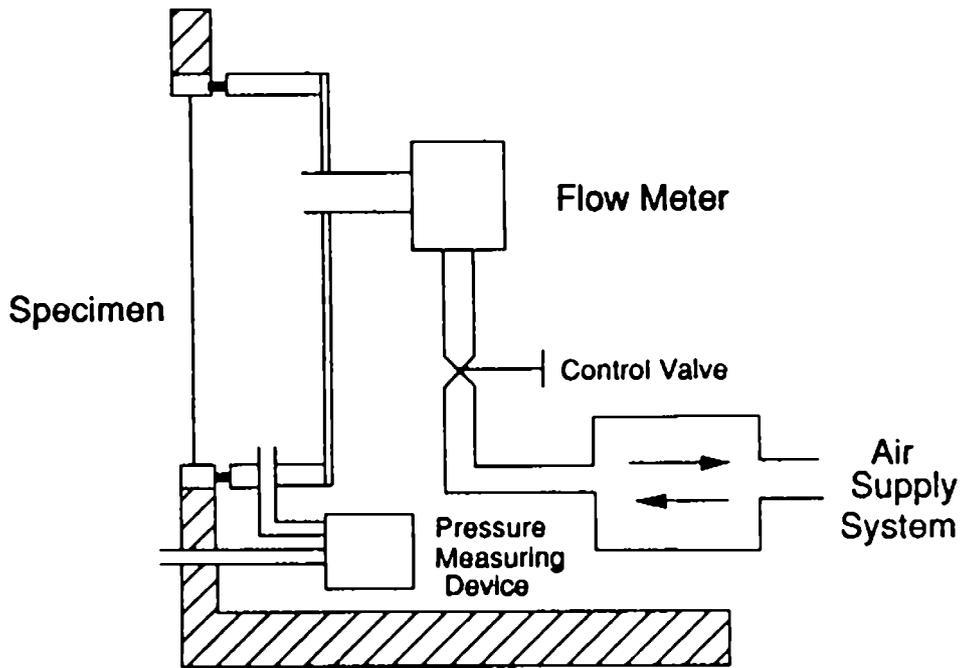
Figure 2. Schematic Layout of Equipment of Component Air Tightness Test Using a Pressurized Enclosure
