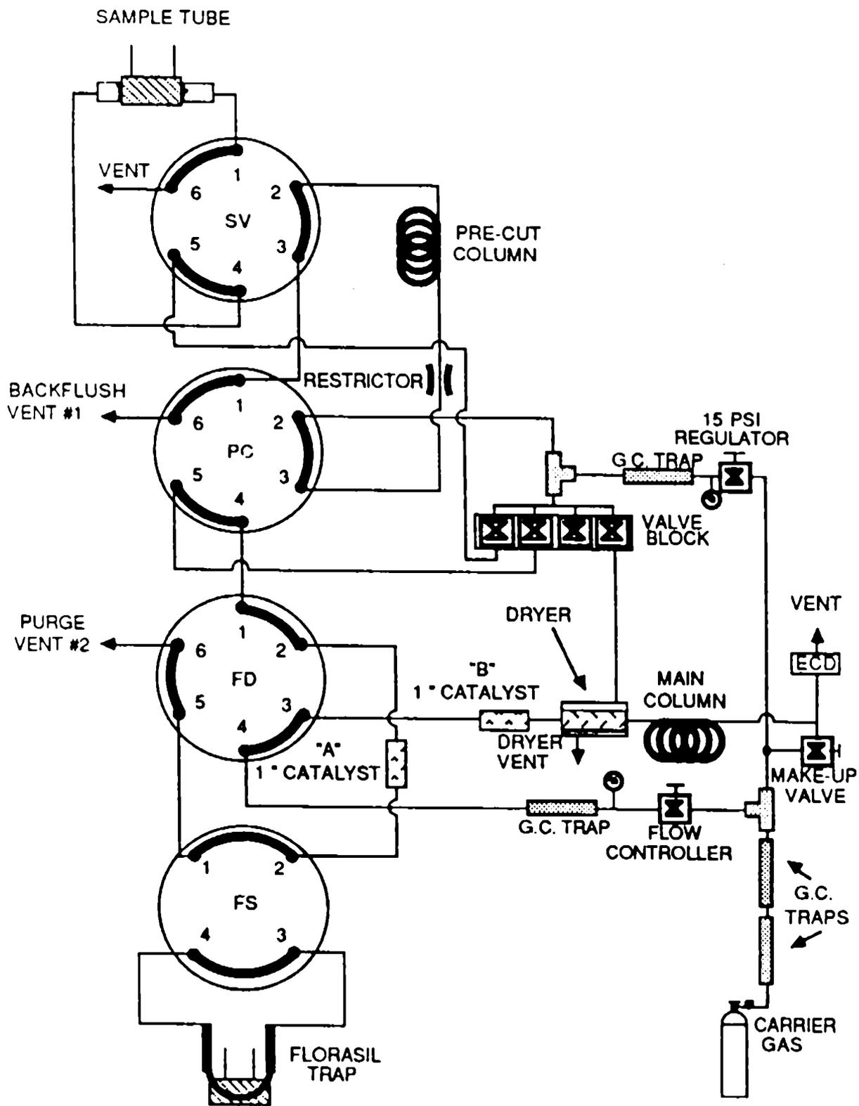
Fig. 6. Schematic of the laboratory GC plumbing. (SV) Sample valve. (PC) Pre-cut column backflush valve. (FD) Flow direction valve to isolate the chromatography occurring in the main column from the loading of the next sample. (FS) Florasil trap valve. All valves are shown in their "off" position.
