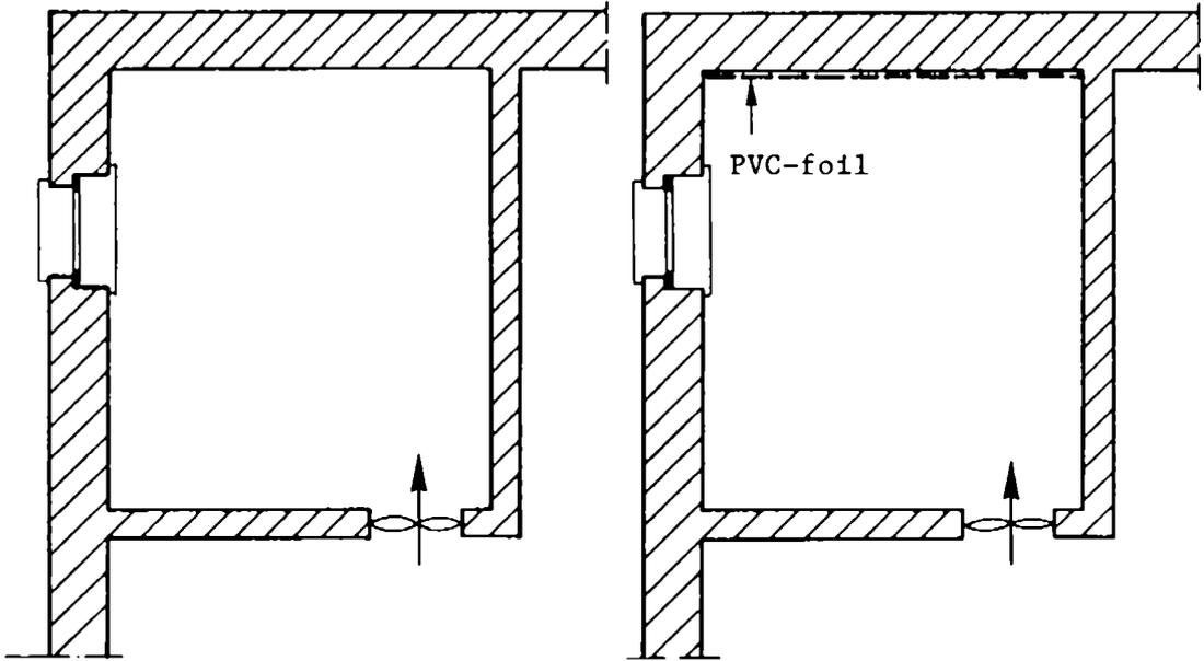
Figure 3.1 - Reference measurement. Figure 3.2 - PVC-foil to make wall airtight.
