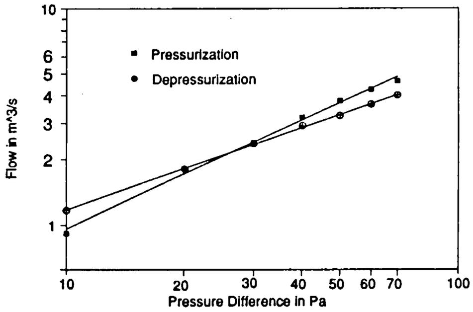
Figure 3. Sample of Air Leakage Graph
