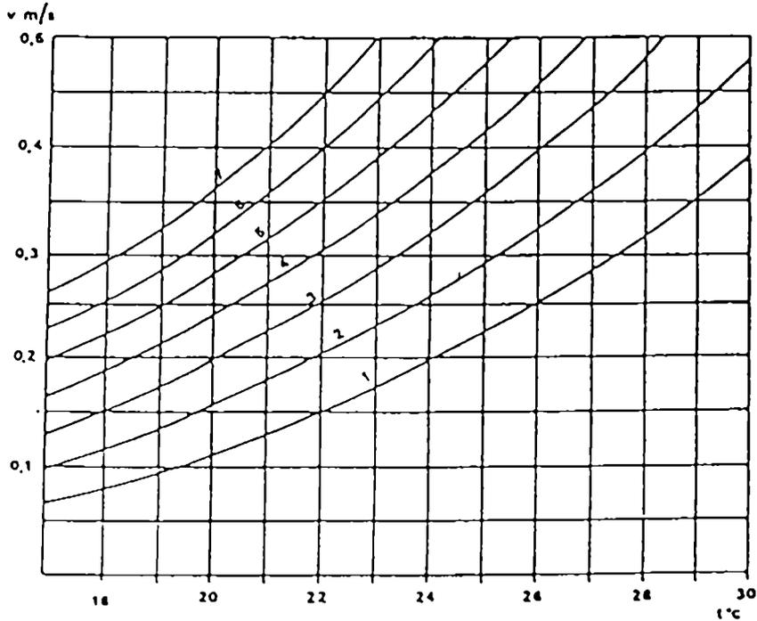
Figure 2. Draught curves for maximum air velocity /2/. Curve 2 is applied for dwelling rooms.
