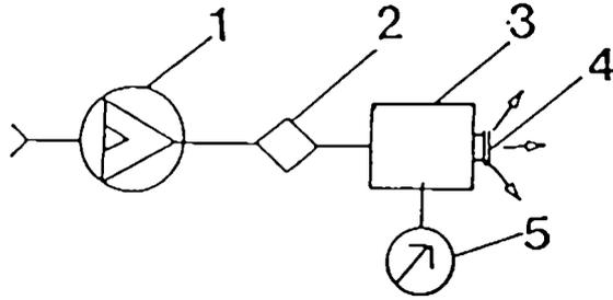
Figure 1. Test arrangement of the air flow rate measurements. /3/
