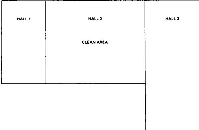
Figure 2: Plan of three hall production area with central clean room. Total area 10,000 m<sup>2</sup>, volume 50,000 m<sup>3</sup>
