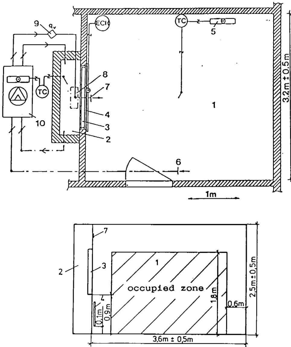
Figure 3. The test room for the draughtlessness tests for the air inlets. /3/
