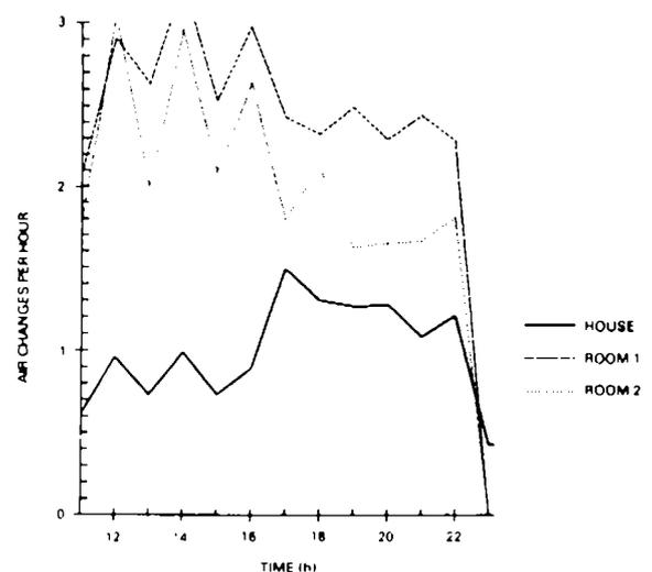
Figure 1: Variation of air change rate with time as measured by CCTG (occupant influence)
